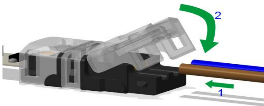
2-1: Insert wire to wire holder of connector and down close cap
